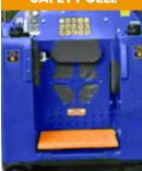
A large operator platform allows for a wider stance, improves safety, and reduces fatigue. A safety cell ensures the operator is enclosed within the operating platform, with side bump protection to provide additional support on rough terrain.
