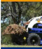
When the bucket is lowered, its ground clearance is the same as the machine. The loader arms can be fully lowered to rest the bucket in its rollback position, aiding when filling, and also transporting material throughout the worksite without load spillage.
